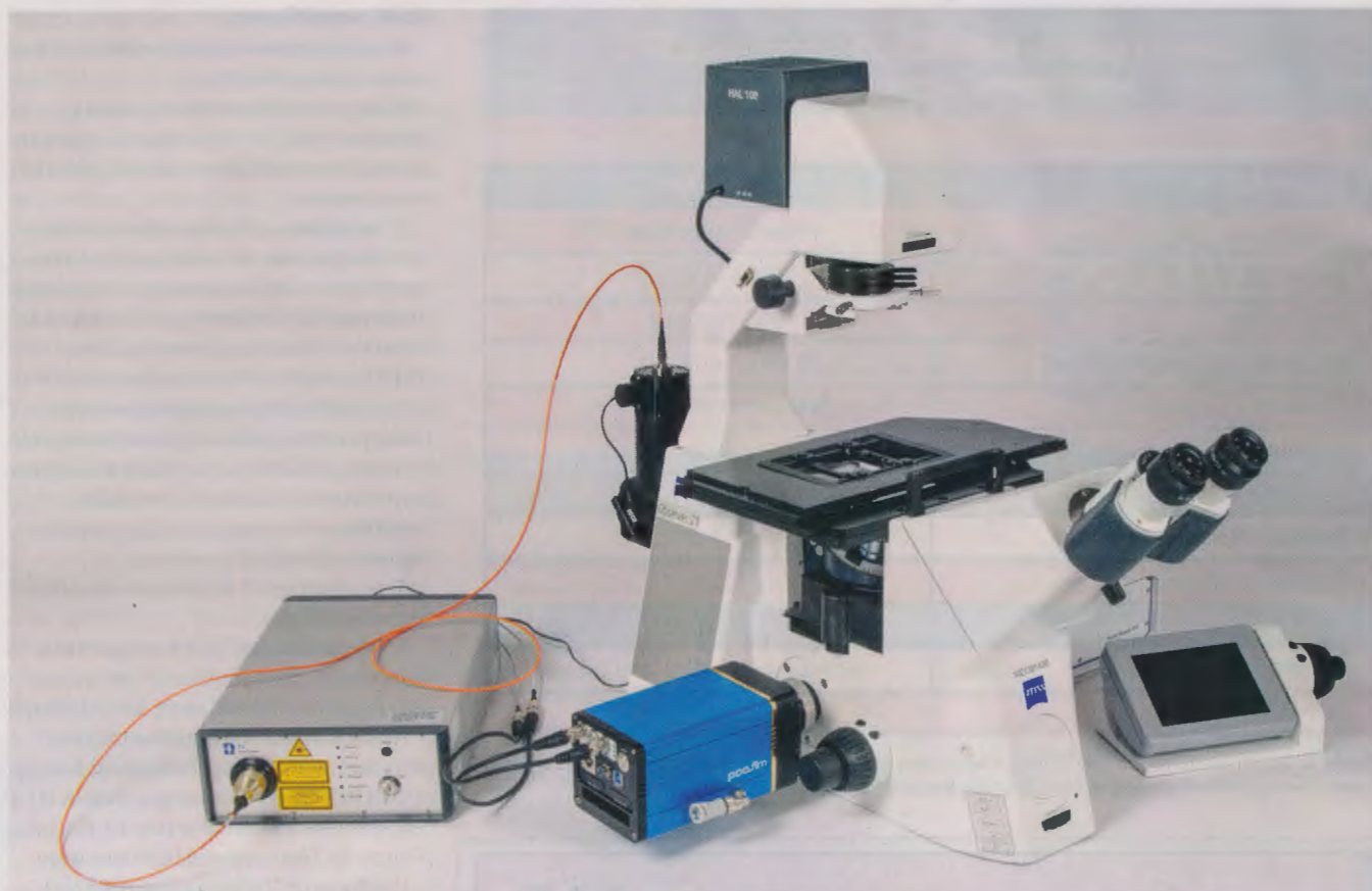
Figure 7. Basic microscope setup for FLIM with the new camera system, pco.flim. From left to right: the laser diode light source (Rapp OptoElectronic), the pco.flim camera system (PCO AG), the optical coupling unit with de-speckling (Rapp OptoElectronic) and an inverse fluorescence microscope (Zeiss AG). Courtesy of PCO AG.
