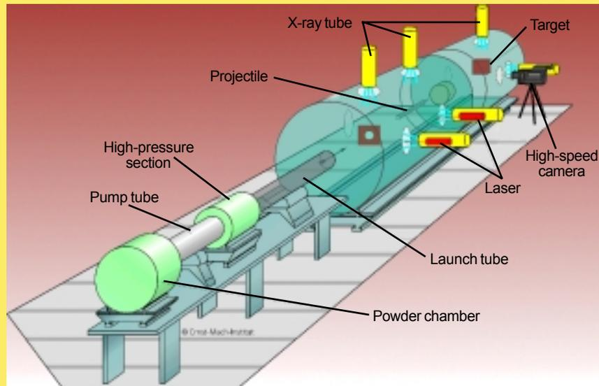
**FIGURE 1.** Typical Ernst-Mach-Institut launch facility is designed to send a projectile into a chamber in which the projectile's impact on a target can be characterized, often with high-speed imaging equipment.
