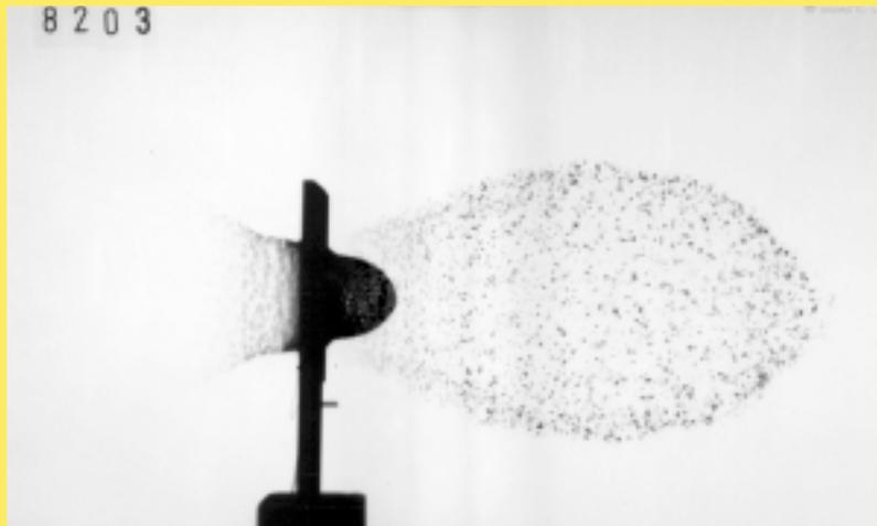
**FIGURE 2.** Double-exposure flash radiography (with a framing sequence of 60  $\mu$ s) images the debris-cloud expansion after impact of an aluminum sphere on a titanium/tungsten shield at 5.7 km/s.
