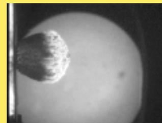
**FIGURE 3.** Ultra high-speed digital imaging captures the impact flash and debris-cloud expansion behind a thin aluminum shield after it is impacted by an aluminum sphere at a striking velocity of 5.2 km/s (framing sequence 5  $\mu$ s, exposure time 20 ns).
