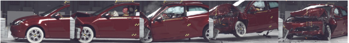
Crashtest, single extracted images of sequence - original resolution 2016 x 2016 @ 1102 frames/s (color version)
