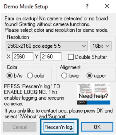
If Camware cannot detect any connected camera, it will start in **Demo mode**. It is also possible to activate **Logfiles** in Demo mode.
