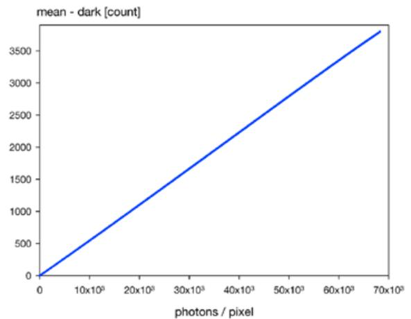
EMVA 1288 linearity measurement of a pco.dimax camera.
