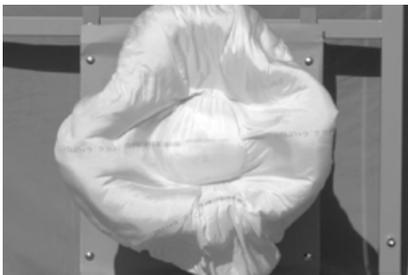
Airbag inflation can be recorded with more than 7000 frames/s at 1k x 1k resolution or with more than 5000 stereo images/s at 1k x 1k resolution (both images in one readout image with mirror set-up).
