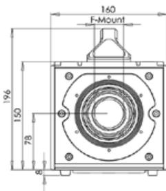
All dimensions are given in millimeter.
