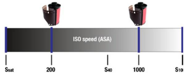
The graph shows the ISO 12232 values  $s_{sat}$ ,  $s_{40}$  and  $s_{10}$  relative to the formerly used sensitivity values for negative film (examples give ASA 200 and ASA 1000) along a virtual sensitivity scale.
